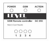
The front panel of GC 055 is equipped with seven LED indicators. The 'Action' LED is controlled by the configuration. The 'GSM' LED indicates the GSM status (Section 7.2).
